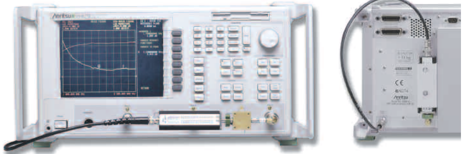
External and internal connections for the Noise Figure measurements choices using Scorpion.
